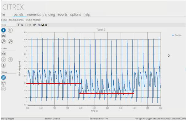
Vsens at 2.0 lpm switched to Psens -3 cmH<sub>2</sub>O and back to Vsens 2.0lpm. Bias flow at red line
