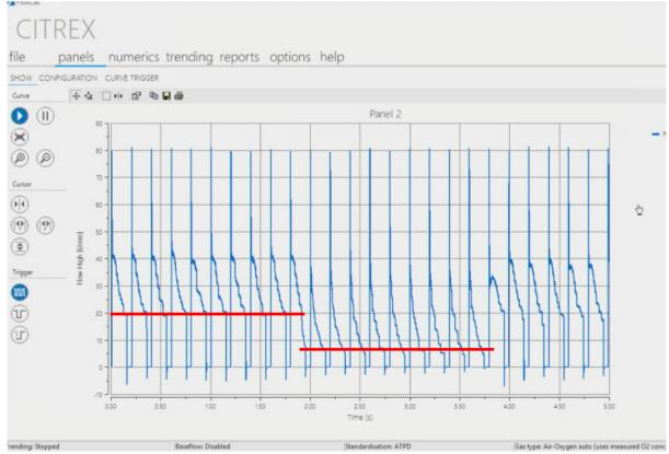
Vsens at 2.0 lpm switched to Psens -3 cmH<sub>2</sub>O and back to Vsens 2.0 lpm. Bias flow at red line
