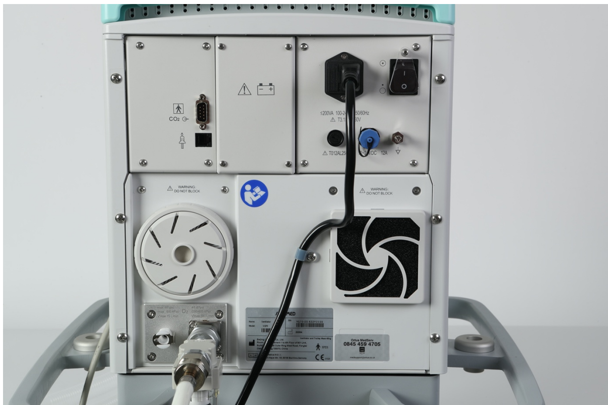
Rear view showing air and piped oxygen inlets
