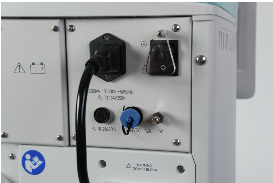
Protected switch at rear shuts machine down without warning
