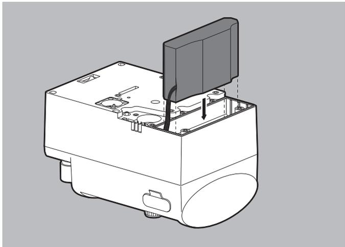
2. Insert the rechargeable battery. Pay attention to the cable routing when doing this.
