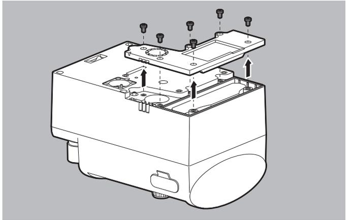
1. Loosen 6 screws from the rechargeable battery compartment cover on the back of the device.
