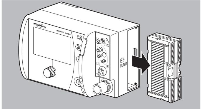
1. Press together and hold the tabs of the locking mechanism.
