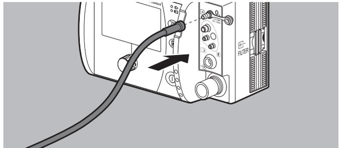
4. Connect the oxygen inlet tube to the device's oxygen inlet.
