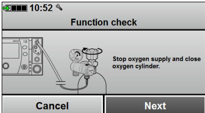
7. Stop the oxygen supply and close the oxygen cylinder
