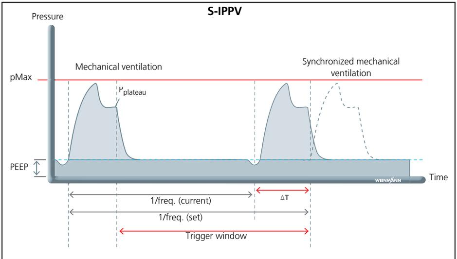
S-IPPV mode is used for volume-controlled ventilation at a variable mandatory minute volume. Throughout the entire expiratory phase, a trigger is active which enables the patient to trigger a new mechanical breath. This means the patient is able to increase his or her respiratory rate – and thus the minute volume – as needed. As a rule, this mode is used on patients who have inadequate spontaneous breathing.
