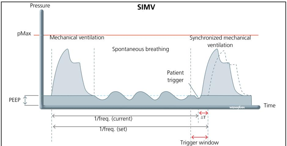
The SIMV mode is used for volume-controlled ventilation at a fixed mandatory minute volume. The patient can breathe spontaneously between the mandatory mechanical breaths and thereby increase the minute volume. During spontaneous breathing, the mandatory mechanical breath is synchronized with the patient's breathing. The mandatory minute volume and the mandatory respiratory rate remain unchanged. The set maximum pressure limit (pMax) ensures the safety of the patient.
