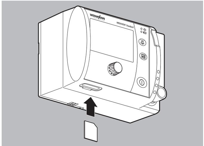
2. Push the SD card into the SD card slot until it clicks into place. When doing so: The beveled corner of the SD card must be at the front on the right during insertion.
