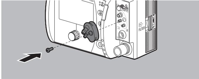
2. Connect the disposable breathing circuit adapter to the ventilation hose connection.
