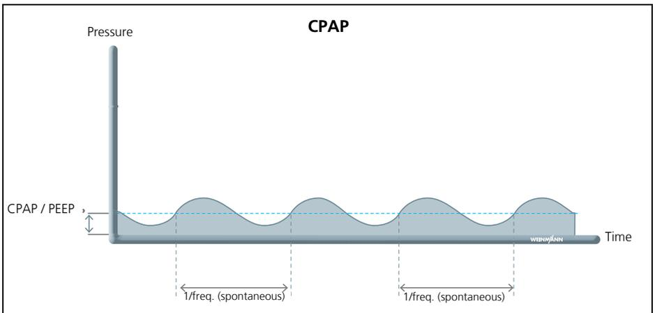
The CPAP / PEEP setting increases the lower pressure level during spontaneous breathing. This results in an increase in the functional residual capacity of spontaneously-breathing patients. The patient is able to breathe spontaneously without any restriction at the set pressure level. The CPAP mode is used exclusively on patients with adequate spontaneous breathing.
