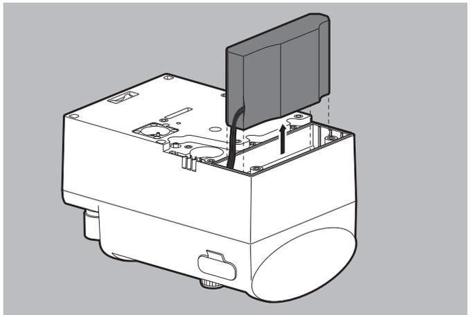
4. Remove the rechargeable battery from the device.
