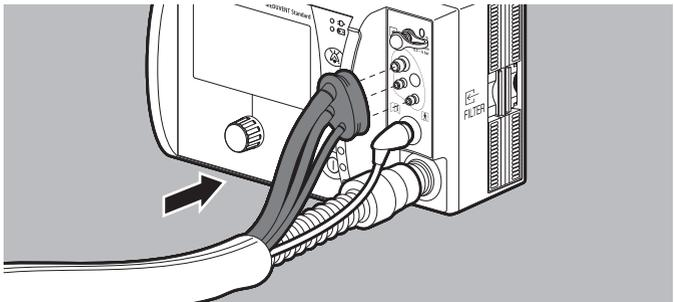
3. Attach the measuring circuit connector to the measuring circuit connection.
