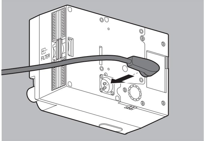
1. Connect the device to line power by its charging adapter (WM 28979) and power supply unit and charger.
