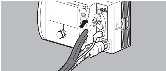
3. Connect the flexible oxygen tube and pressure measuring tube.
