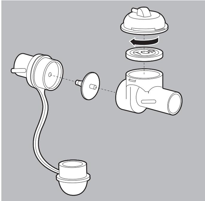
1. Attach the band of the protective cap to the check valve diaphragm holder.
