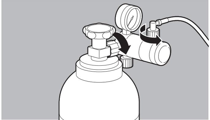
2. Connect the pressure reducer (see "14.2 Accessories and other parts", page 133) to the oxygen cylinder valve using a fluted union nut and tighten it by hand.
