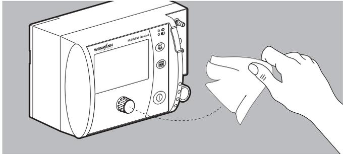
5. If the cleaning and disinfection plan stipulates that parts have to be wiped down: Wipe down parts using a clean, lint-free disposable cloth moistened with cleaning solution.
