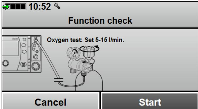
5. Set the oxygen supply rate (5-15 l/min)
