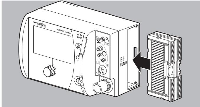
1. Push the hygiene filter into the filter compartment until the hygiene filter audibly engages and is flush with the device.
