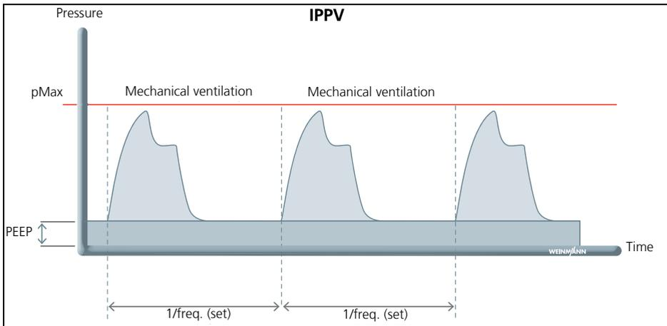
IPPV mode is used for mandatory, volume-controlled ventilation at a fixed tidal volume. This mode is used on patients who have no spontaneous breathing. However, a spontaneously breathing patient can breathe deeply and freely during expiration. The set maximum pressure limit (pMax) ensures the safety of the patient.
