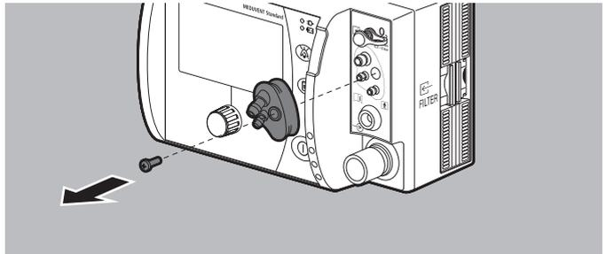
1. Loosen the screw on the disposable breathing circuit adapter.
